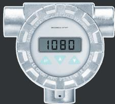
**FRD:** Field Mounted, Loop Powered Indicator - Can be externally mounted anywhere within power loop. Epoxy Coated Aluminum or 316 SS Class1, Div1, Group B, C, D
