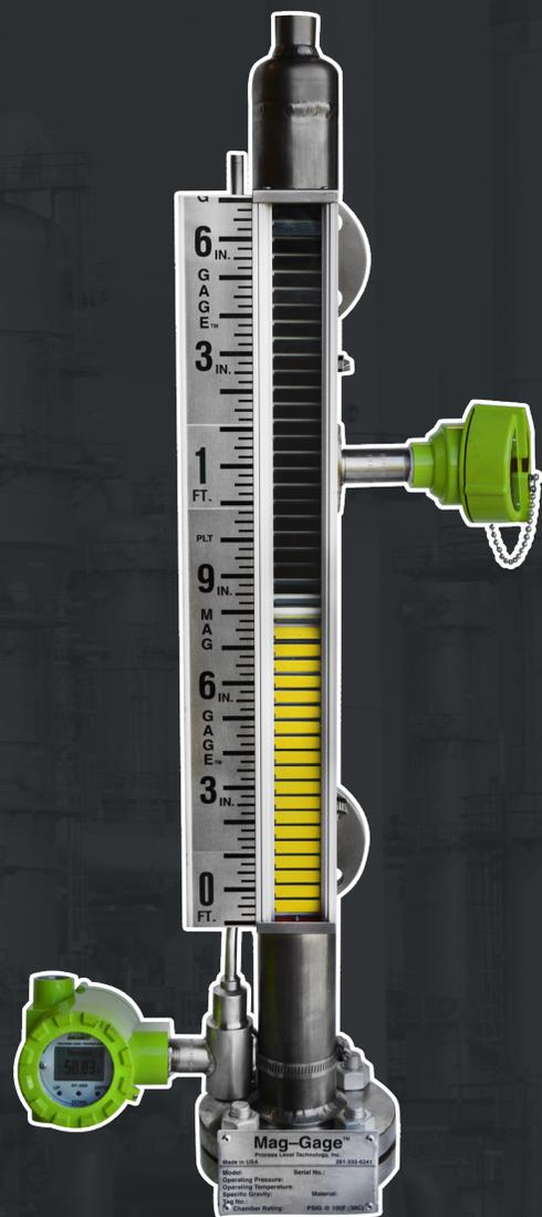
The Process Level Technology Mag-Gage® is a proven method to measure liquid levels. The Mag-Gage® is one of the safest and most economical ways to measure and control your level requirements. It can be installed on almost any shape, size or type of vessel in the industry. In applications of extreme pressure, temperature, vibration and highly corrosive or hazardous material the Mag-Gage® will perform where others fail.
